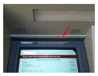
This is an example of a bar camera that is placed right above the screen. Notice that there is a color difference compared to other parts of this ATM, however, the screen frame and unit color is not the same either. The arrow is pointing to the small camera eye.
