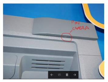
**Pin Camera** – This is an example of a camera that could be attached to a through-the-wall, walk-up or drive-up unit. There is a color difference in this example, and it is bumped out from the actual machine fascia. To a member us the machine for a withdrawal, something like this is likely to be overlooked unless they are more familiar with the aesthetics of a machine.
