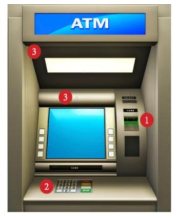
1. **Card Reader** – Overlay card skimmers/readers can be placed and removed quite quickly and easily, check your card readers daily by pulling gently. On the contrary, deep insert card readers are not detectible by the eye because they are completely inserted into the card reader.
